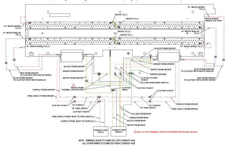
\*\*Note - Basic Schematic, including reed switch. Dimming leads, surge protection device and EM option not shown here.\*\*
